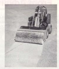
Engaging and disengaging attachments is a quick, simple operation using two securing pins. A full range of non-powered accessories is available to make the Jaden Loader indispensable, do-it-all worker essential on every site. Carry-all self levelling platforms, forks, blades, buckets and rippers can be interchanged to complete a hundred jobs with the one machine.
