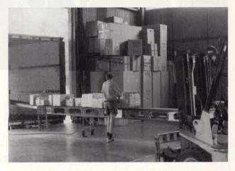
Portable conveyors from Conveyor & Hoist Rentals are used to load freight on to a truck at Australian Road Express
